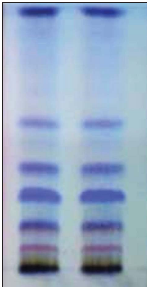
Fig. III. Chloroform extract of Stem bark Solvent system: Toluene: Ethyl acetate (9 : 1)
